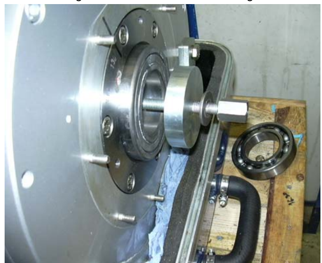
Fig. 7.10.1.3-6: Put on ball bearing
