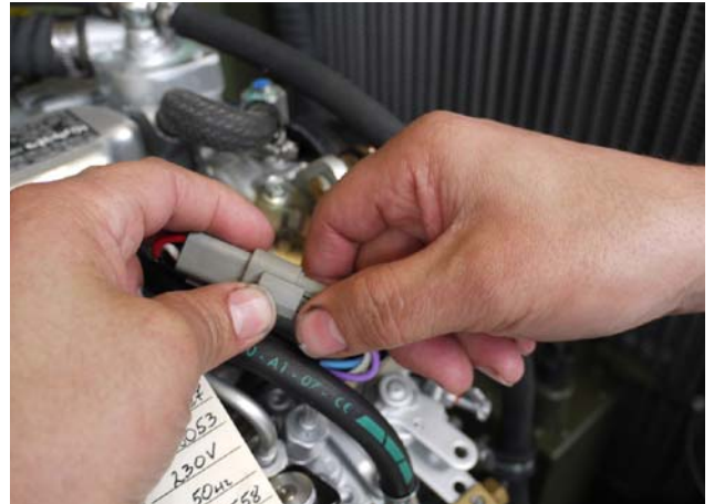
Fig. 7.21-3: Stop solenoid
