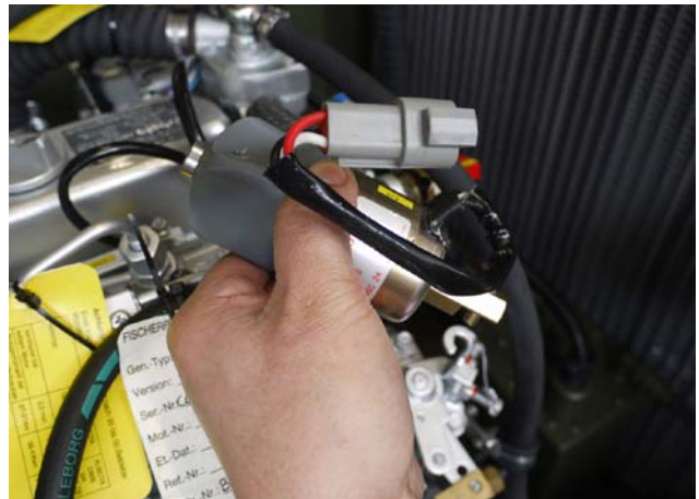
Fig. 7.21-6: Stop solenoid
