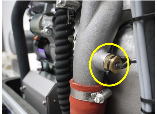
Fig. 4.2.4-5: Thermo-sensor fresh water out
