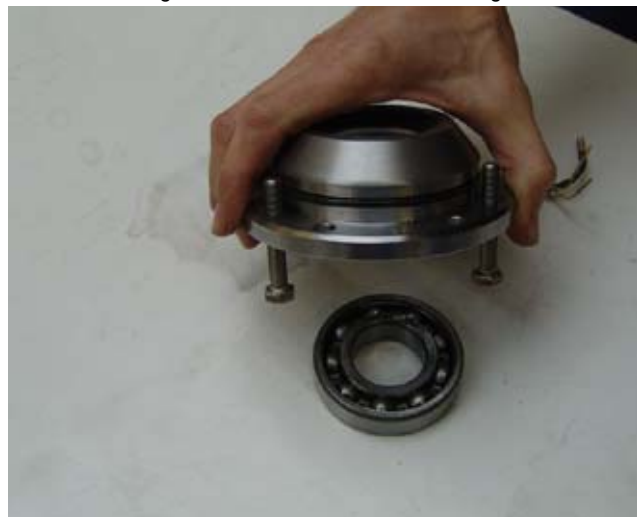
Fig. 7.11.2-10: Dismount the shaft sealing ring
