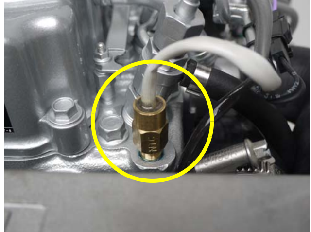
Fig. 4.2.4-2: Coil thermo-switch
