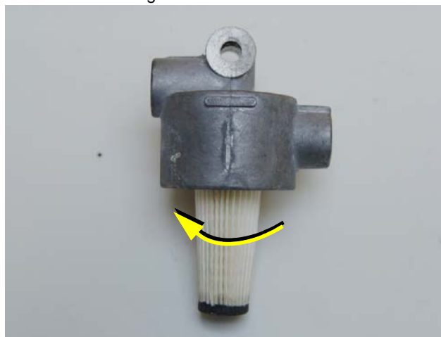
Fig. 7.12.1.1-4: Fuel filter
