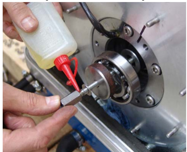
Fig. 7.11.2-27: Mounting the ball bearing
