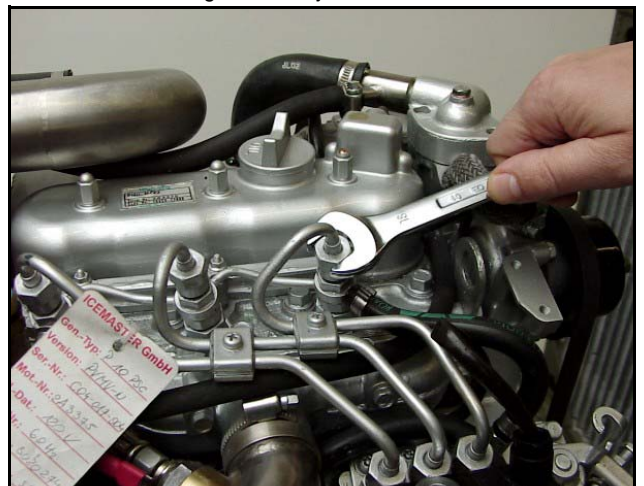
Fig. 7.12-3: Injection nozzles
