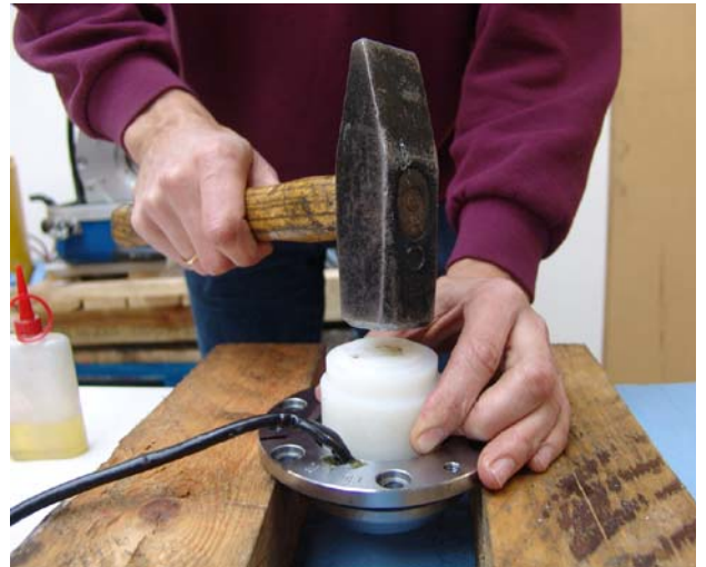
Fig. 7.11.2-17: Fitting the shaft sealing ring
