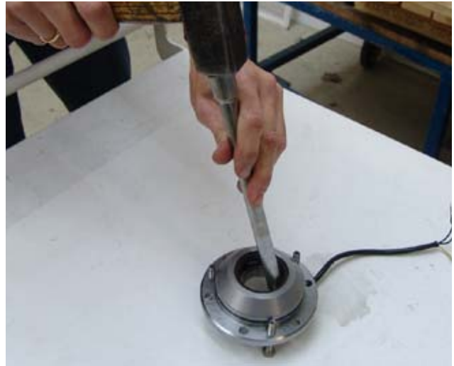
Fig. 7.11.2-9: Dismounted ball bearing
