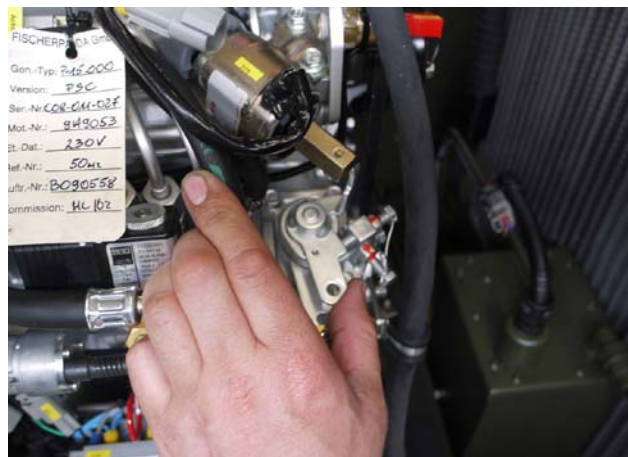
Fig. 7.21-9: Stop solenoid
