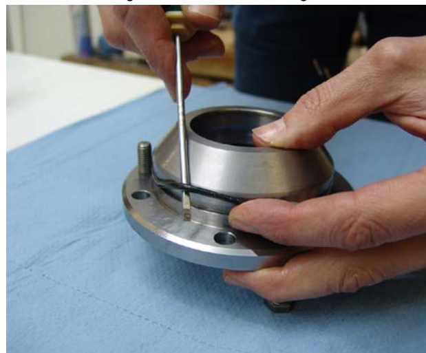
Fig. 7.11.2-12: Remove o-rings
