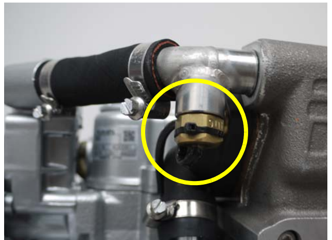
Fig. 4.2.4-6: Oil pressure switch
