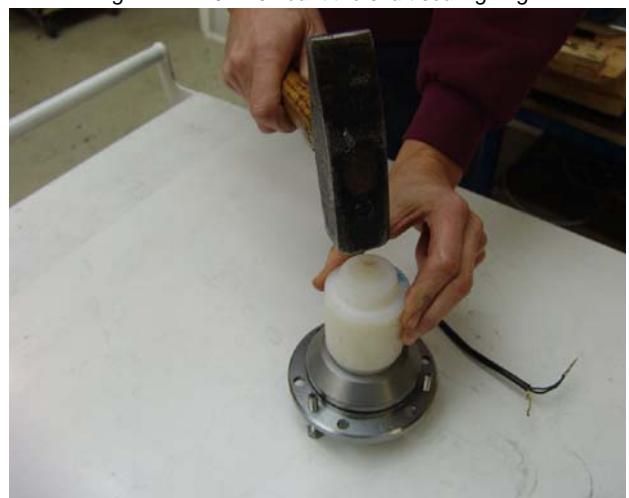
Fig. 7.11.2-10: Dismount the shaft sealing ring
