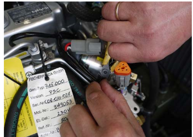
Fig. 7.21-4: Stop solenoid
