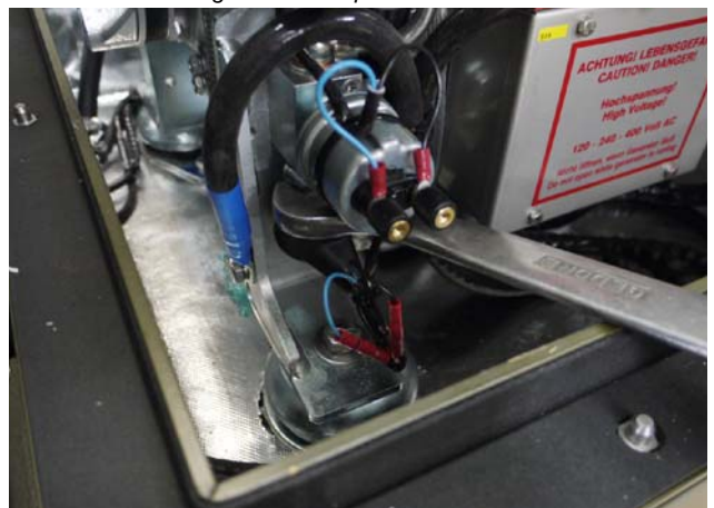
Fig. 7.19-2: Oil pressure sensor
