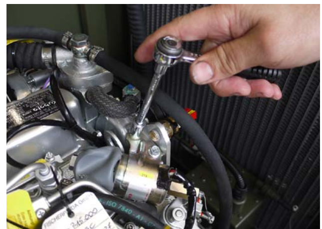
Fig. 7.21-5: Stop solenoid
