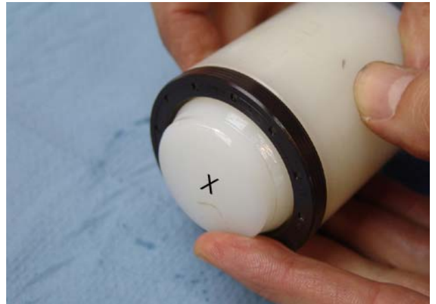
Fig. 7.11.2-17: Fitting the shaft sealing ring
