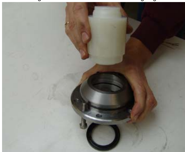
Fig. 7.11.2-12: Remove o-rings
