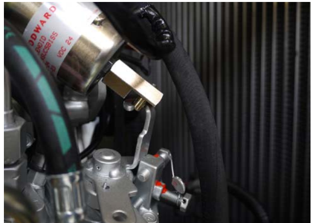
Fig. 7.21-8: Stop solenoid
