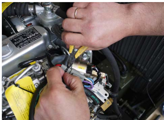
Fig. 7.21-2: Stop solenoid
