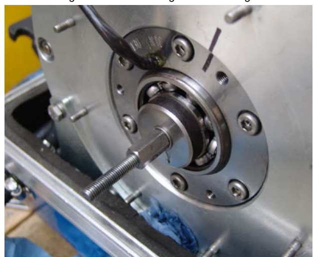
Fig. 7.11.2-27: Mounting the ball bearing
