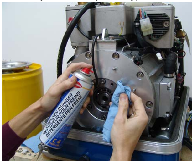
Fig. 7.11.2-4: Marking the bearing position
