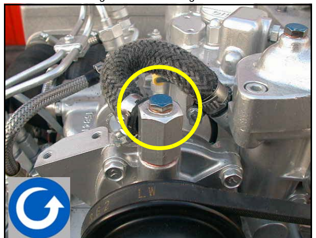
Fig. 7.13-2: Ventilating screw
