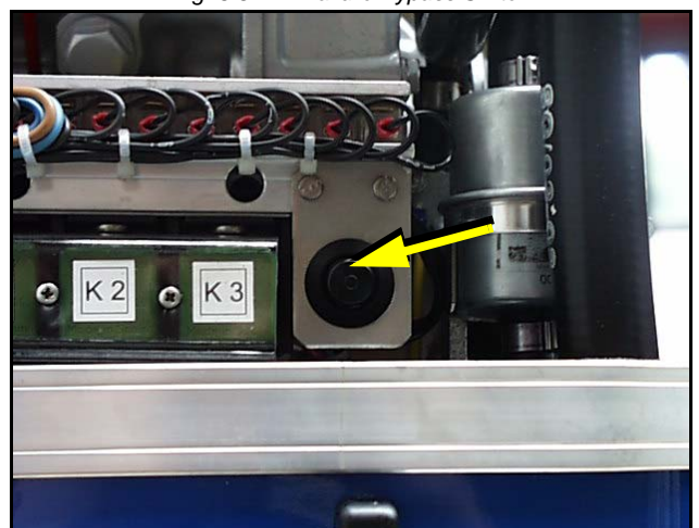
Fig. 8.8.2-1: Failure Bypass Switch
