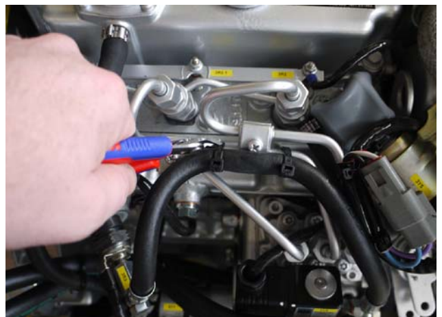
Fig. 7.20-1: Injection nozzles
