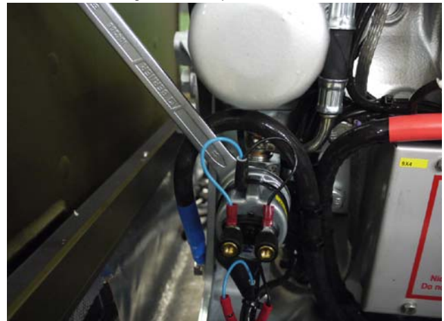
Fig. 7.19-2: Oil pressure sensor
