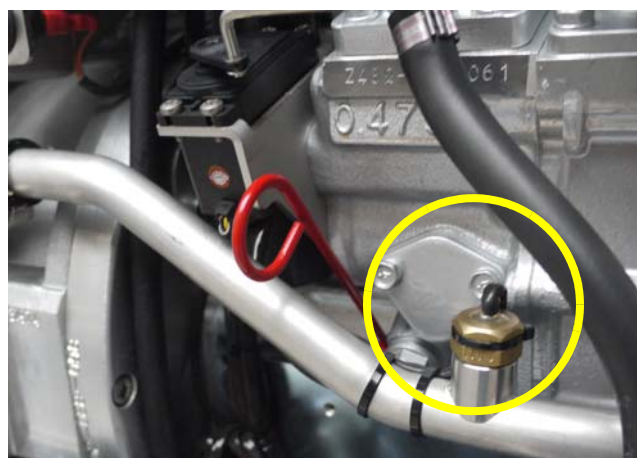
Fig. 4.2.4-3: Thermo-sensor raw water in
