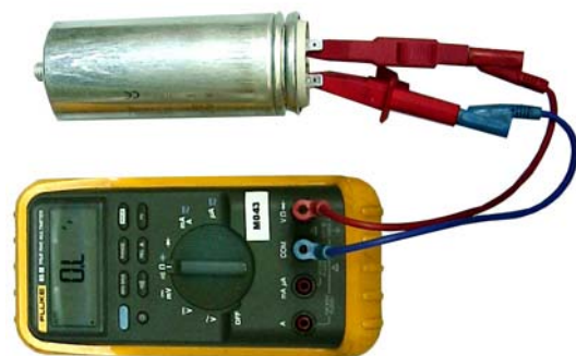
Fig. 7.17.2-3: Capacitor checking
